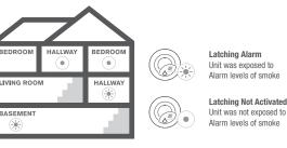
This Alarm includes "Smart Interconnect" which enables the Alarm to be interconnected with other First Alert® Smoke, Heat, and "Smart Interconnect" CO Alarms. When smoke is detected, all Alarms will sound the smoke horn nattern. When CO is detected, "Smart Interconnect" Alarms will sound the CO horn pattern Alarms that do not have the "Smart Interconnect" feature will remain silent during a CO Alarm.
